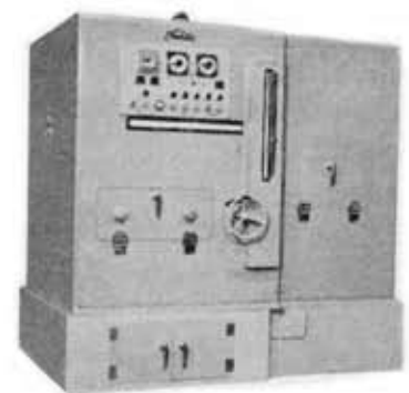
The 2-kCi 137 Cs \gamma -ray irradiator specially designed for seed, Model RE-1017
